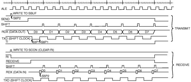
Figure 1.23. Serial Port Mode 1. TCLK, RCLK, and Timer 2 are present in the 80C32/80C52, 80C154/83C154 and 83C154D.
