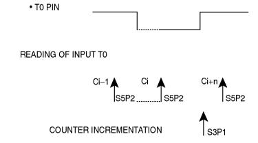
The counter will only evolve if a level 1 is detected during state S5P2 of cycle Ci and if a level 0 is detected during state S5P2 of cycle Ci + n.
