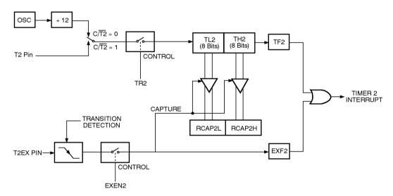
In the auto-reload mode there are again two options, which are selected by bit EXEN2 in T2CON. If EXEN2 = 0, then when Timer 2 rolls over it not only sets TF2 but also causes the Timer 2 registers to be reloaded with the 16-bit value in registers RCAP2L and RCAP2H, which are preset by software. If EXEN2 = 1, then Timer 2 still does the above, but with the added feature that a 1-to-0 transition at external input T2EX will also trigger the 16-bit reload and set EXF2.
