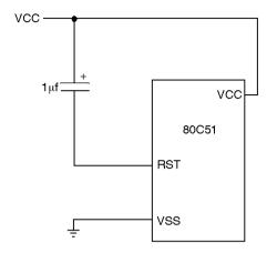
A reset accomplished by holding the RST pin high for at least two machine cycles (24 oscillator periods), while the oscillator is running. The CPU responds by executing an internal reset. It also configures the ALE and PSEN pins as inputs. (They are quasi-bidirectional). The internal reset is executed during the second cycle in which RST is high and is repeated every cycle until RST goes low. It leaves the internal registers as follows:
