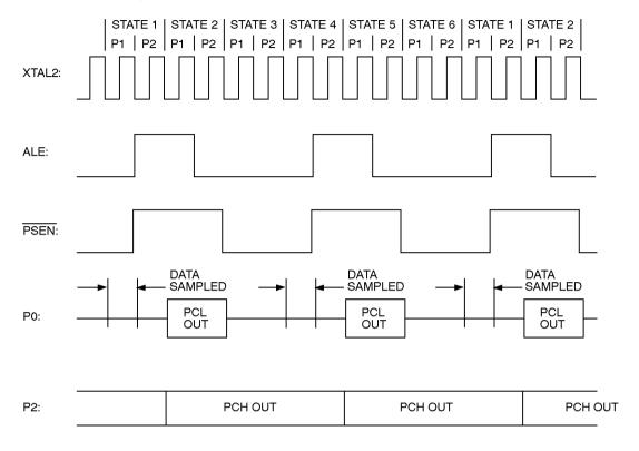
Figure 1.37. External Data Memory Read Cycle.
