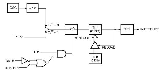
Figure 1.15. Timer/Counter 0 Mode 3: Two 8-bit Counters.
