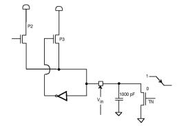
The figure 1-9 shows the behaviour of the port during 0-to-1 transition.
