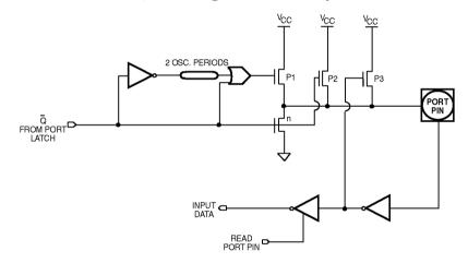
CMOS Configuration. pFET 1 is turned on for 2 osc. periods after Q makes a 1-to-0 transition. During this time, pFET 1 also turns on pFET 3 through the inverter to form a latch which holds the 1. pFET 2 is also on.
