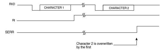
In this example the character 1 is received and the RI bit is set to 1. A second character is sent before the CPU reads the first one. The character 1 is overwritten and SERR bit is set to 1 to indicate the loss of the first character.
