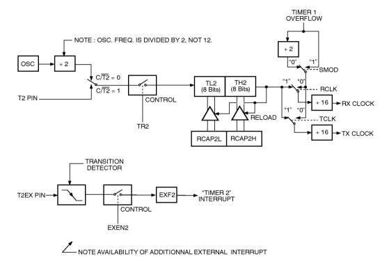
The baud rate generator mode is similar to the auto-reload mode, in that a rollower in TH2 causes the Timer 2 registers to be reloaded with the 16-bit value in registes RCAP2H and RCAP2L, which are preset by software.
